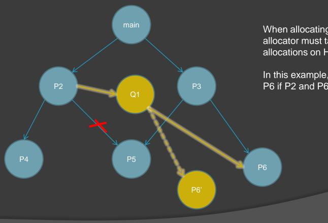
When allocating register for Q1, allocator must take care of existing allocations on HARD micro-code
