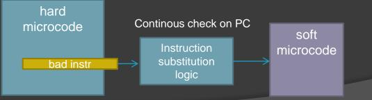
Execution flow is transferred to SOFT area after matching instruction address Address spaces are contiguous, code on SOFT area can jump back to HARD area
